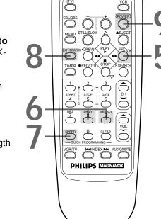
**Press the SPEED button to select the tape speed.** The selected tape speed, SP or SLP, will appear beside REC SPEED.
